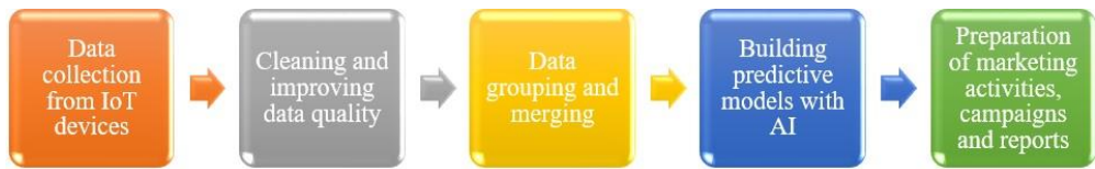
Figure 4: The IoT data processing system submodules
